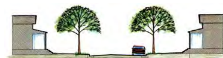
20.12m (66 ft.) ROW for local streets with sidewalk and landscaping areas on both sides
