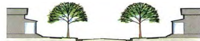
25m (82 ft.) ROW for collector streets allowing for sidewalk both sides, boulevard and on-street parking
